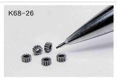
We produce Small Module Gear for AV equipments, amusement machines, and so on. The gear module is 0.15 to 0.30. We developed new press machine, special powder material, and high accuracy die, for realize Small Module Gear by powder metallugy technique.
